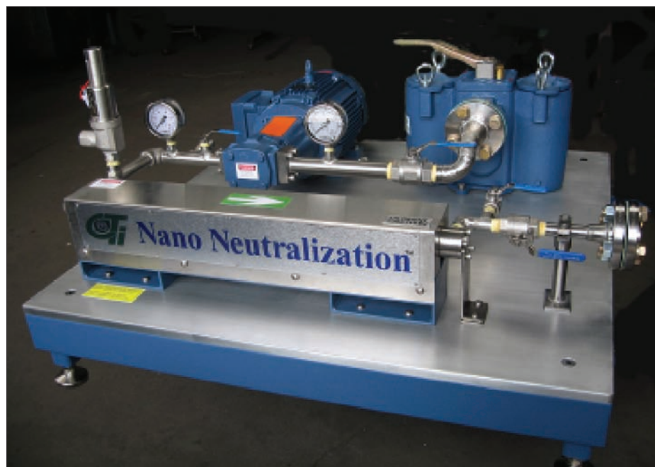
A NANO REACTOR FOR A LOW CAPACITY NANO NEUTRALISING PLANT OF <200 TONNES/DAY
